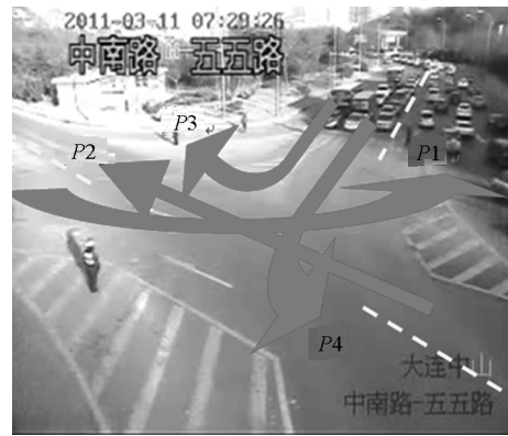
图 7 初始方向为多路口的四种轨迹模式场景 Fig. 7 Four kinds of trajectory models of initial direction for crossing situation
