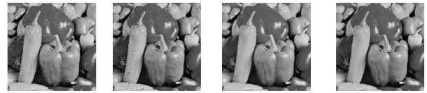
(u) \gamma_{(B_1,B_1^c)} 结果 (u) The result of \gamma_{(B_1,B_1^c)} (v) \varphi_{(B_1,B_1^c)} 结果 (v) The result of \varphi_{(B_1,B_1^c)} (w) (\varphi\gamma)_{(B_1,B_1^c)} 结果 (w) The result of (\varphi\gamma)_{(B_1,B_1^c)} (x) (\gamma\varphi)_{(B_1,B_1^c)} 结果 (x) The result of (\gamma\varphi)_{(B_1,B_1^c)}
