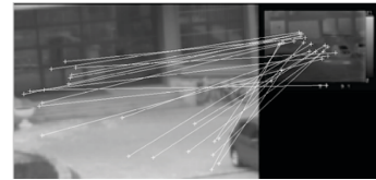
(b) 去除多对一映射的候选同名点对 (b) Corresponding point pairs after removing “N-1 mapping”
