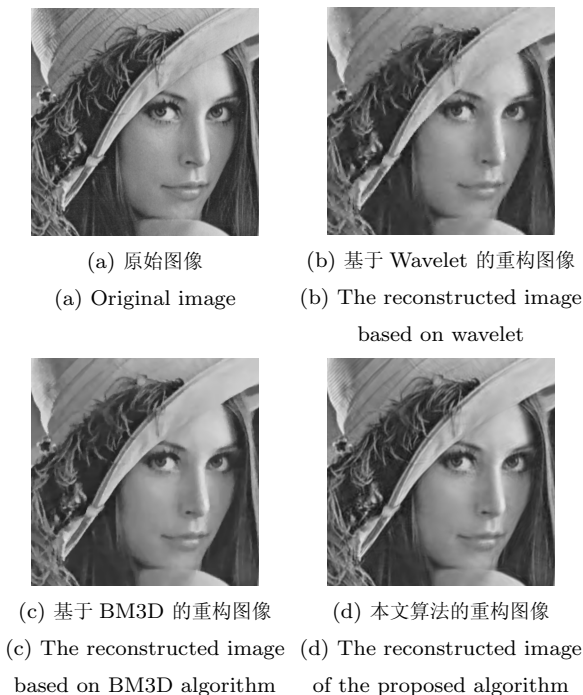
图 6 20% 抽样率时 Lena 图像的重构结果 Fig. 6 The reconstruction results of the Lena image (Sample ratio is 20%.)
