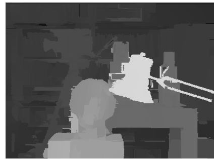
图 4 采用基于投票的平面拟合方法得到的视差图 Fig. 4 The disparities obtained by the plane fitting algorithm based on voting
