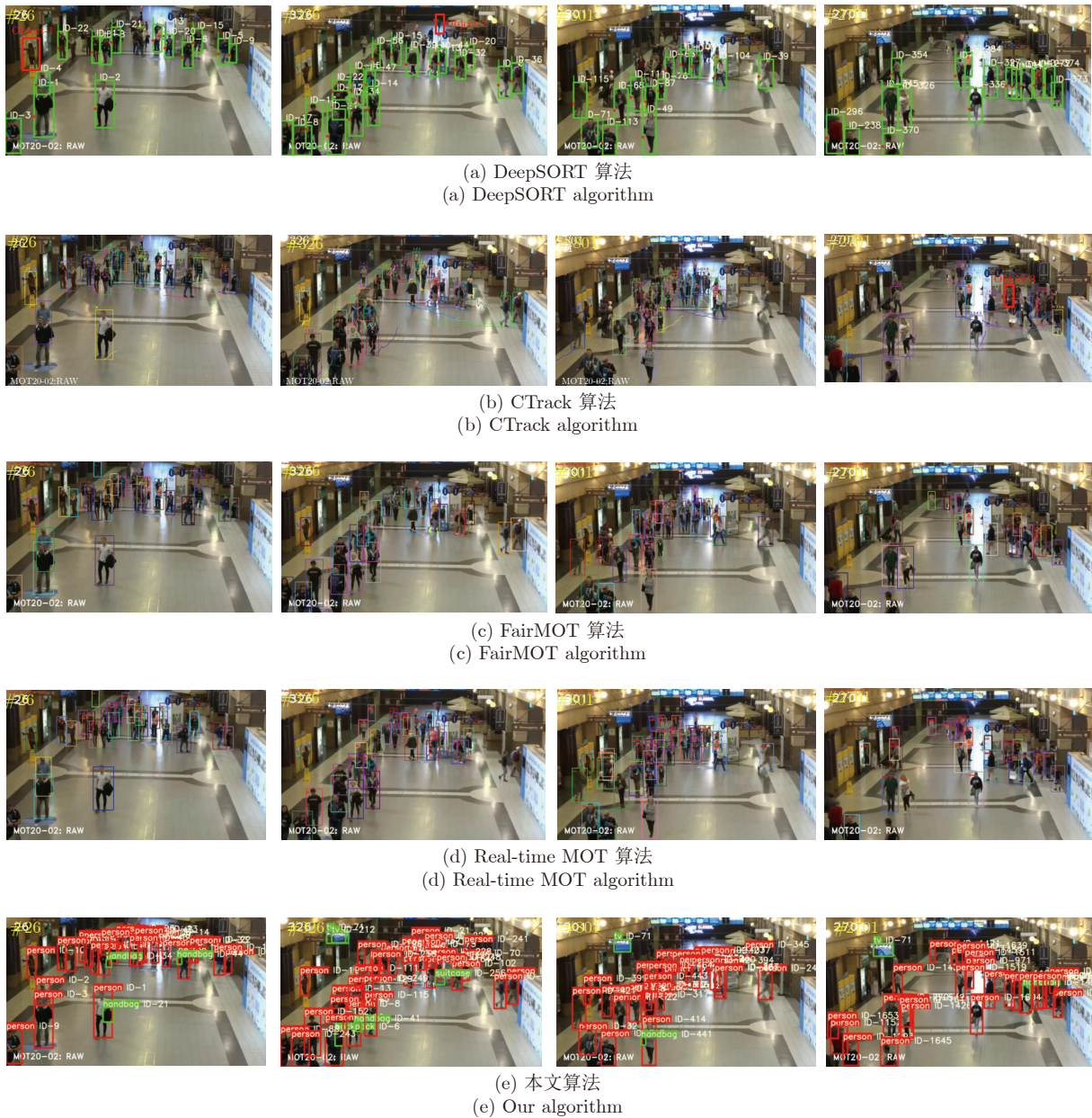
图 8 本文算法与 DeepSORT、CTrack、FairMOT、Real-time MOT 多目标跟踪算法对比分析 Fig.8 Comparison and analysis of our algorithm with DeepSORT, CTrack, FairMOT, and Real-time MOT multi-target tracking algorithm
