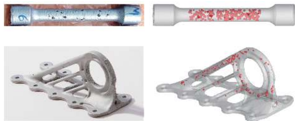
图 2 拉伸杆和航空工件原图像及 CT 重建的三维图像 Fig.2 Original images of stretching rods and aerial parts and three dimensional images rebuilt by CT
