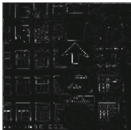
(b) 传统小波在四个方向的处理结果之和 (b) Sum of the results from all level 2 traditional wavelet transform filtering
