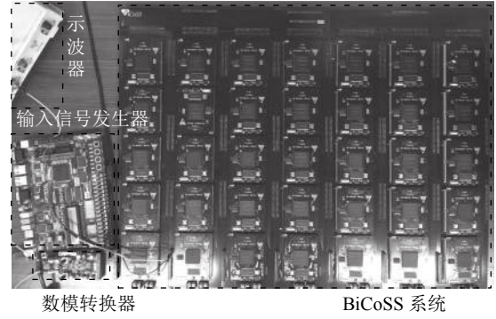
(a) 基于 BiCoSS 系统的类脑计算平台实物图 (a) Brain-inspired computing platform based on BiCoSS system
