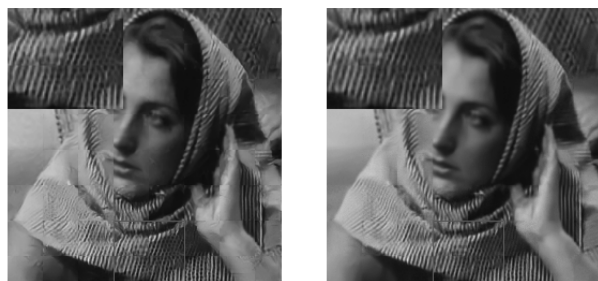
(a) 修正前 PSNR = 26.69 dB (a) PSNR = 26.69 dB before refined (b) 修正后 PSNR = 27.53 dB (b) PSNR = 27.53 dB after refined
