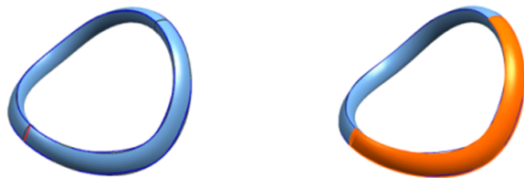
(b) 焊缝模型非理想几何特征的自动识别 (b) Automatic identification for nonideal geometric features in a weld model of steel frame
