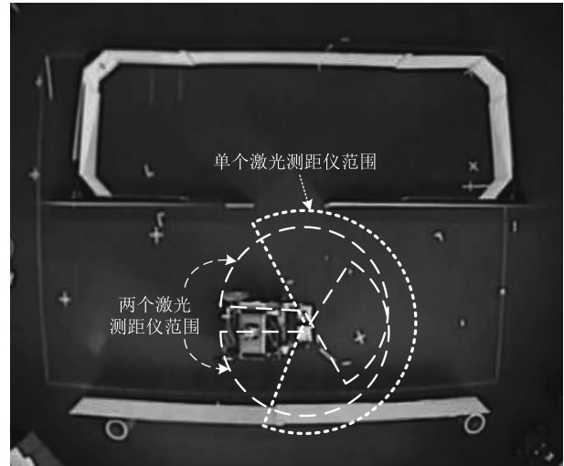
图 14 两个激光测距仪相对于单个的优势 Fig. 14 Advantage of two lasers compared with single laser
