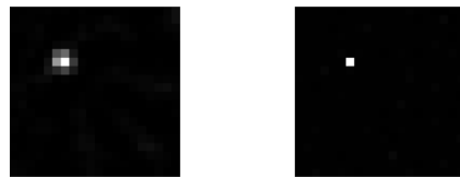
(a) 吉洪诺夫正则化方法 (b) l_1 范数正则化方法 (LASSO 算法) (a) Simulations of Tikhonov regularization method (b) Simulations of l_1 -norm optimization method
