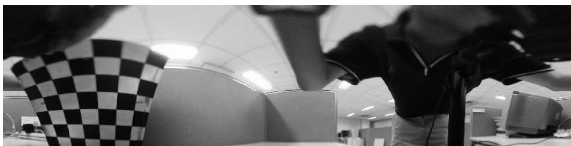
Fig. 9 A panoramic image generated with the calibrated intrinsic parameters of our method
