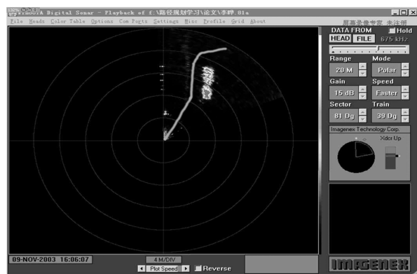
图 3 AUV 小范围海区的路径规划 Fig. 3 Small region path planning by AUV
