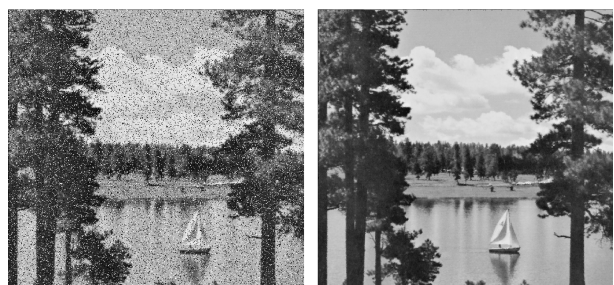
图 4 15% 椒盐噪声污染的 Sailboat 图像及滤波后结果 Fig. 4 Sailboat image corrupted by 15% salt & pepper noise and the filtering result
