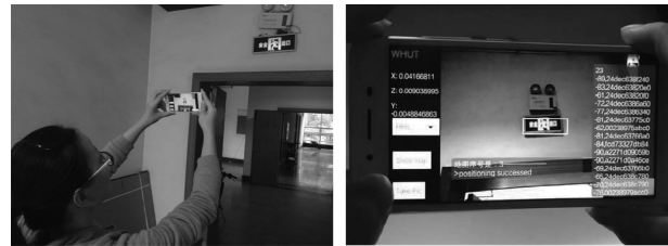
(a) 利用智能手机拍摄消防安全出口标志 (a) Use the Android application to shoot the exit sign (b) 将消防安全出口标志置于候选框内 (b) Put the sign in a white selection window on the image
