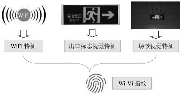
图 1 WiFi 与视觉相融合的定位指纹 — Wi-Vi 指纹 Fig. 1 WiFi and vision integrated positioning fingerprint — Wi-Vi fingerprint
