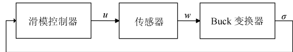
图 4 Buck 变换器滑模控制系统的等价变换 Fig. 4 Equivalent block diagram of sliding mode controlled Buck converter system
