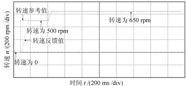
(c) 电机低速调速波形
