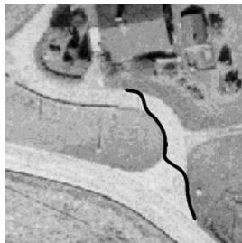
(b) 传统 Snake 方法提取效果 (b) Extraction effect of traditional snake
