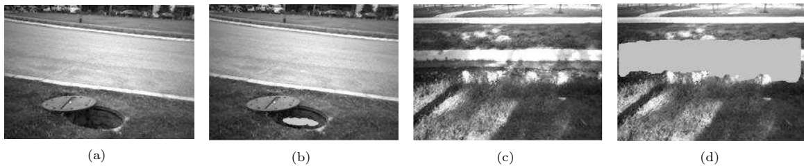
Fig. 7 The negative obstacle (water well) and its detection results in different scenarios ((a) and (c) The original right images; (b) The obstacle detection result of (a); (d) The obstacle detection result of (c). The obstacle is indicated by a high-lighting region.)
